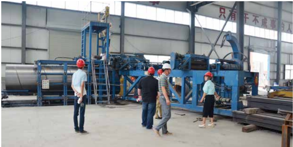
DN600-1600mmX6000mm PCCP Steel Cylinder welder
