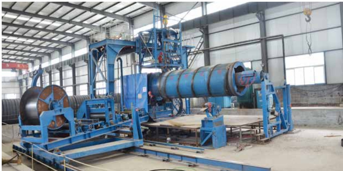
DN1400-3600mmX6000mm PCCP Steel Cylinder welder
