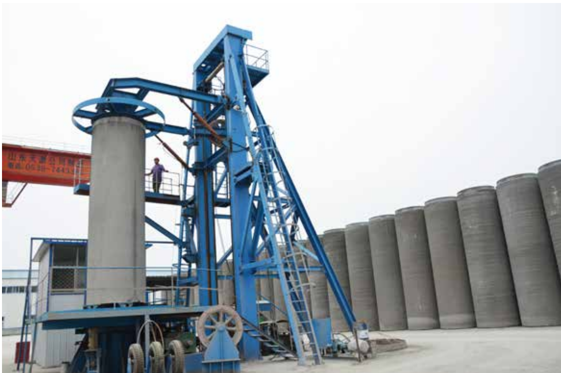
Vertical PCCP Pipe Steel Wire Wrapping Machine
